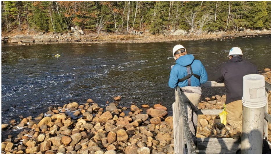
Photo 3.7 Gaging below the Gorham dam using the ADCP drone boat
