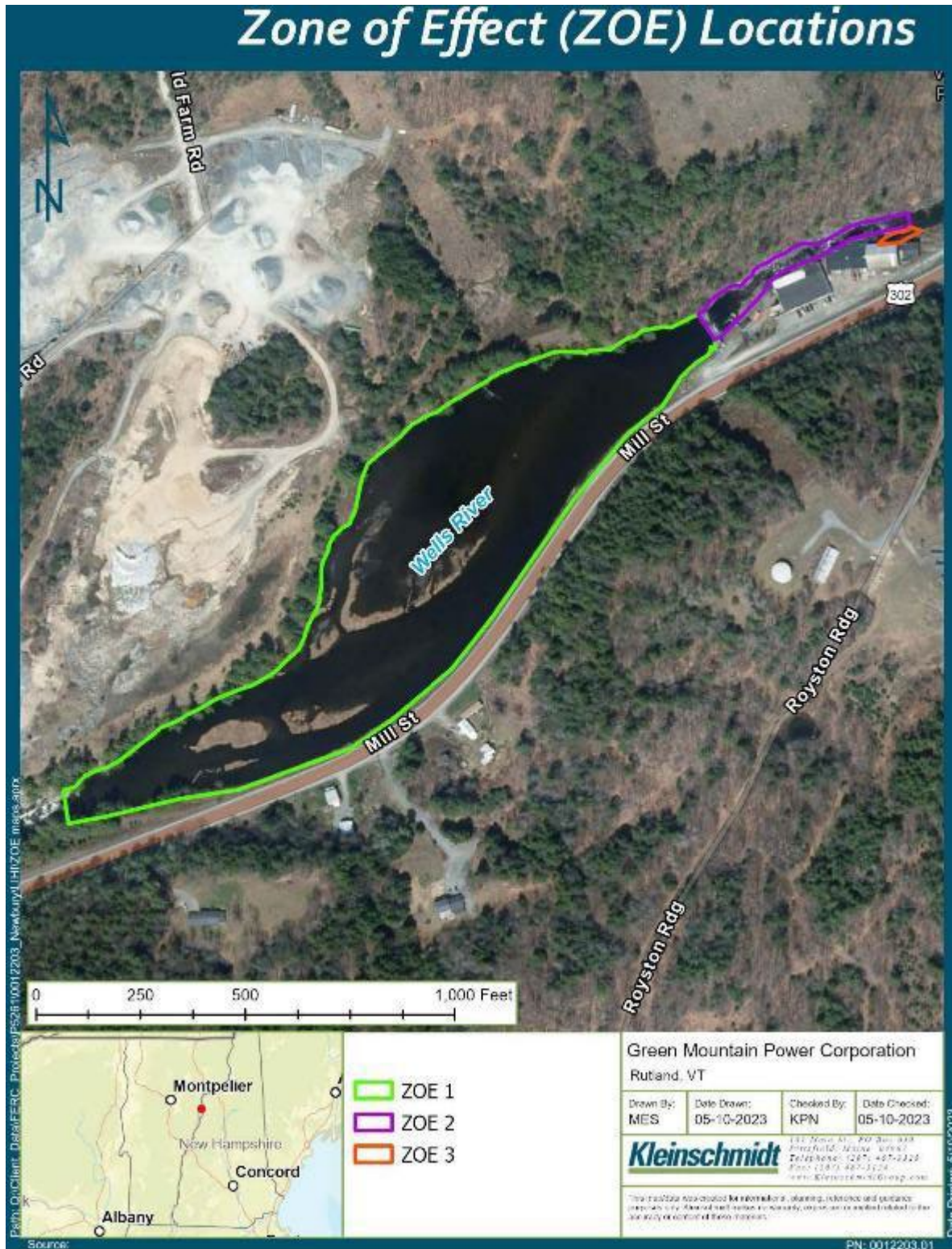
Figure 6. Newbury Hydroelectric Project's ZOE map. Green = ZOE 1 Impoundment, Purple = ZOE 2 Bypass, Orange = ZOE 3 Tailrace.
