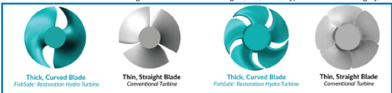
Figure 3. Natel RHT Blade Designs (blue) versus typical turbine blades (gray) 3 .
