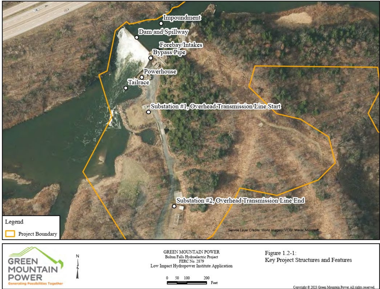
Figure 2. – Photograph of Bolton Falls Project (aerial) showing the Impoundment, Dam, Bypassed Reach, Powerhouse, and Tailrace.
