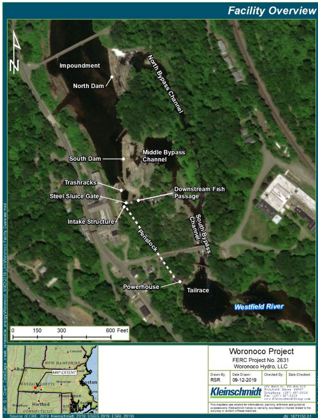
Figure 3 - Key Features of the Woronoco Project
