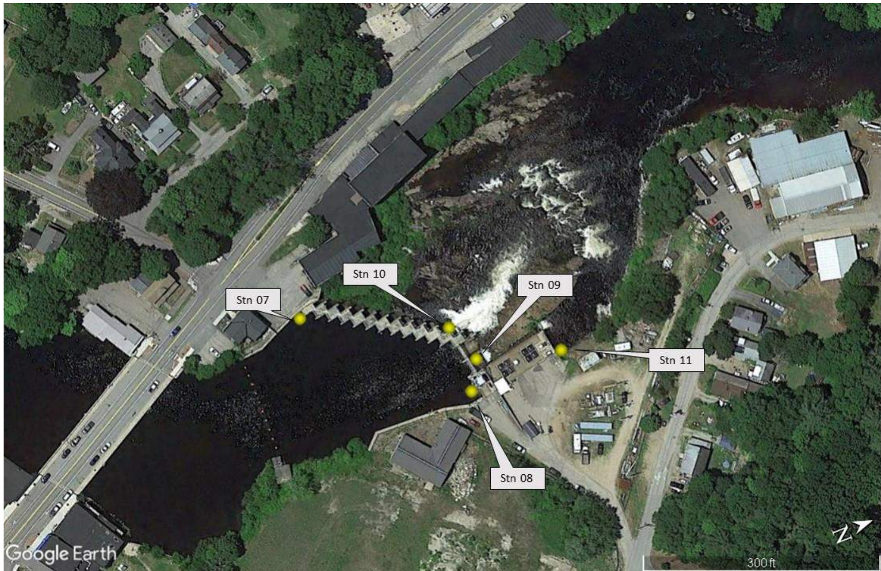
Figure 60–2. Final stationary receiver placement at PUF for the adult river herring downstream passage study, May 24 – June 30, 2021.
