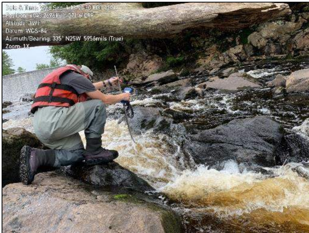
Figure 29–5. Measuring depths and velocities at potential migration barriers in the Rolfe Bypass reach.
