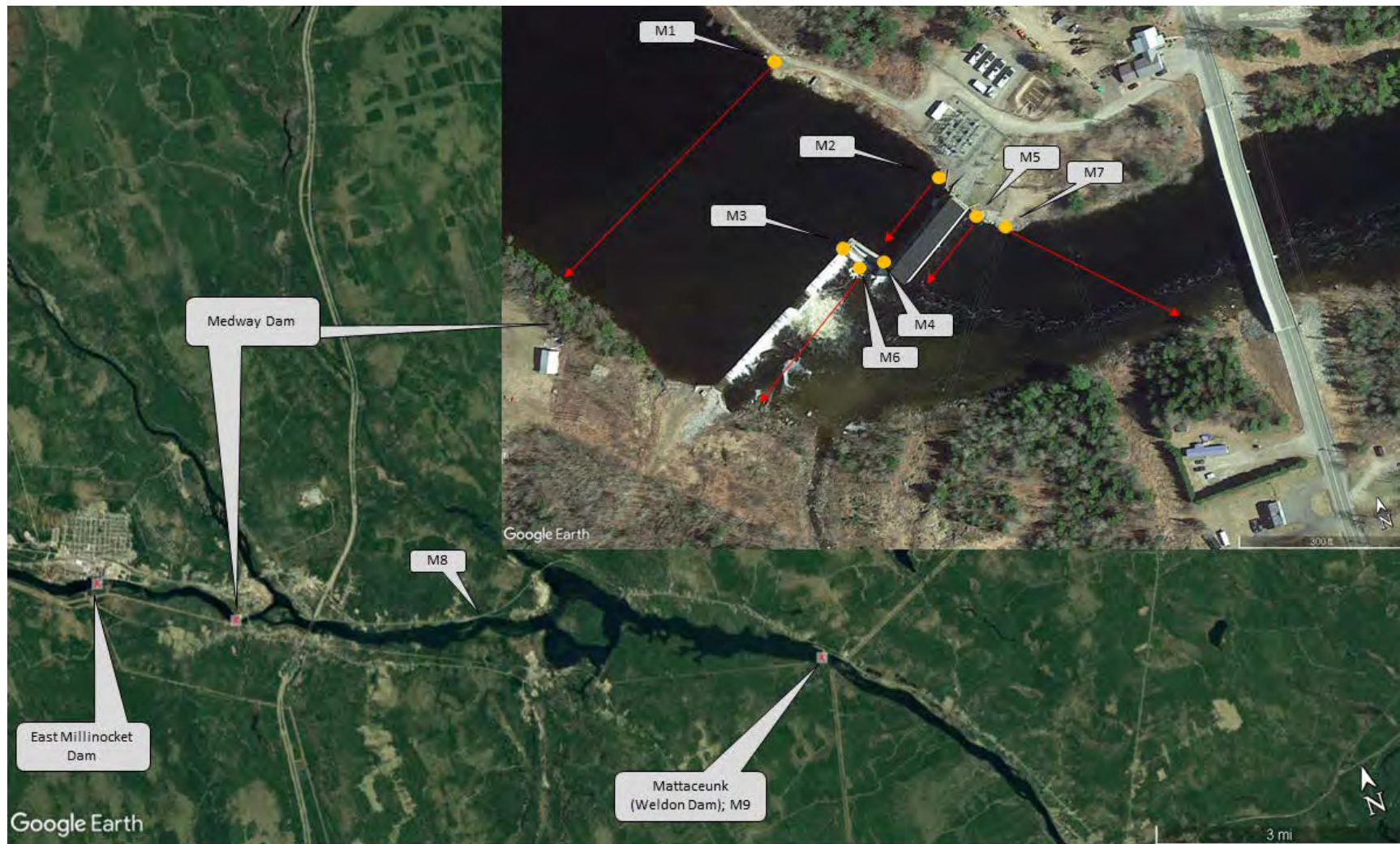
Figure 3–1. Approximate locations and coverage areas for Monitoring Stations installed for evaluation of downstream passage of adult American eels at Medway during 2020.
