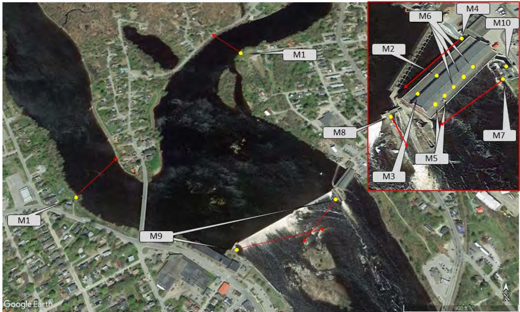
Figure 3–2. Locations for Monitoring Stations M1-M10 during the 2020 juvenile alosine downstream passage route evaluation study at Milford.
