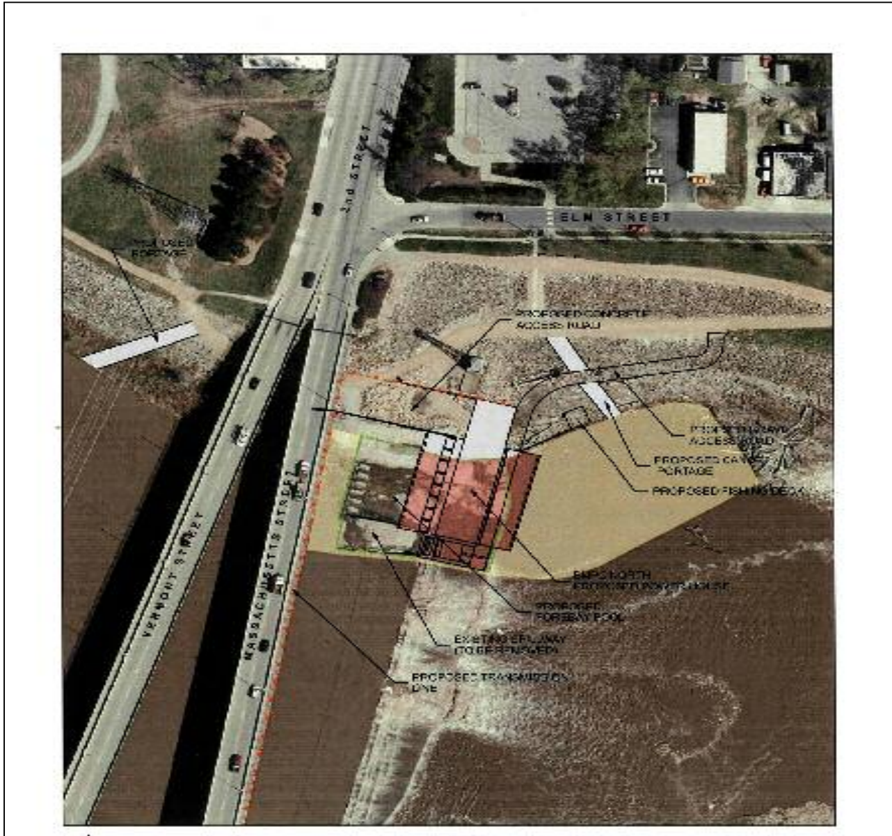
Figure 2. General layout of project facilities at the proposed north powerhouse (Source: Bowersock 2010a).
