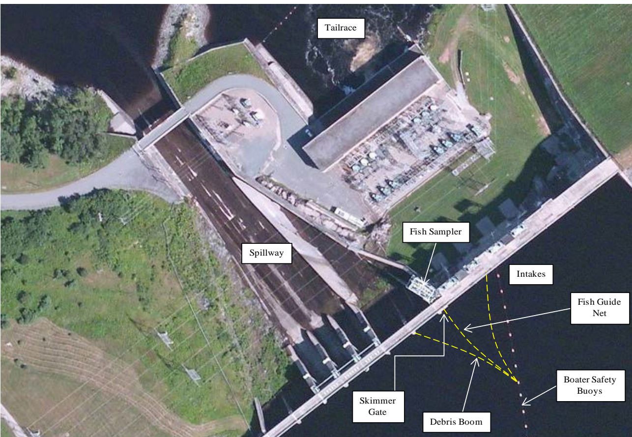
Figure 1-3. Schematic of the Moore Dam Development showing the guide net used during 2009 and 2010 studies and its relation to the fish sampler, hydroelectric turbine intakes and tailrace.
