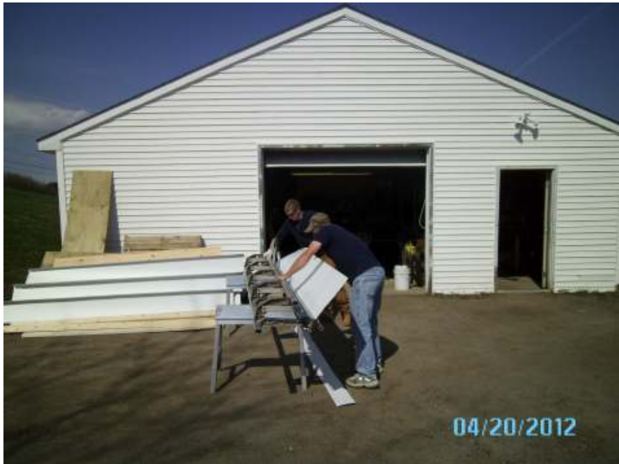
Powder coated aluminum trays being formed.
