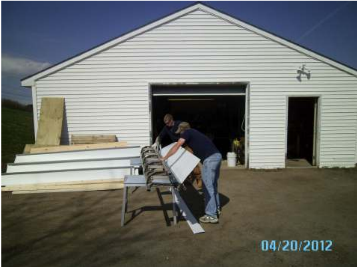
Powder coated aluminum trays being formed.
