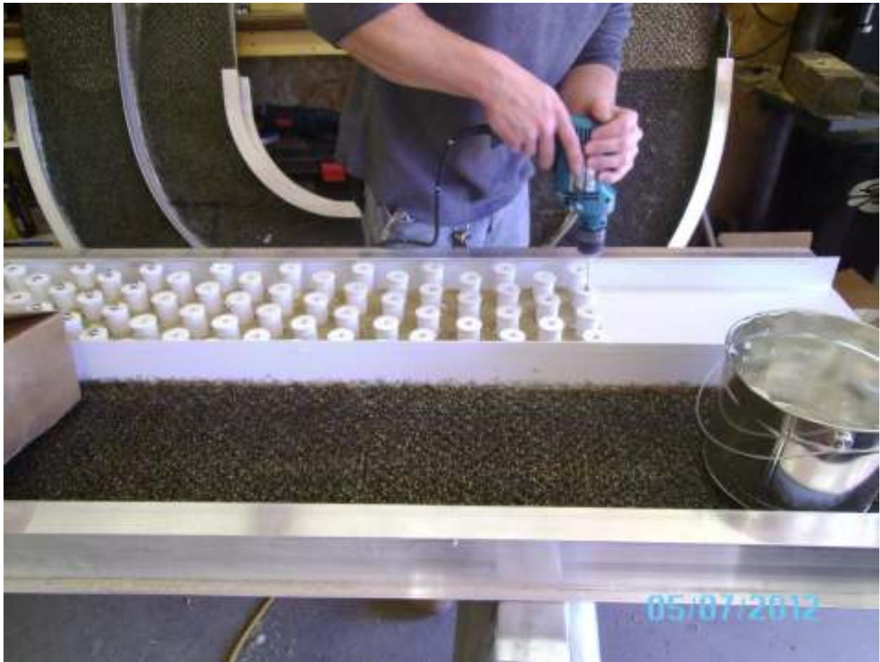
Assembling of staggered peg tray. In the view above the Enkamat covered tray can be seen in place as well as the partition between trays.
