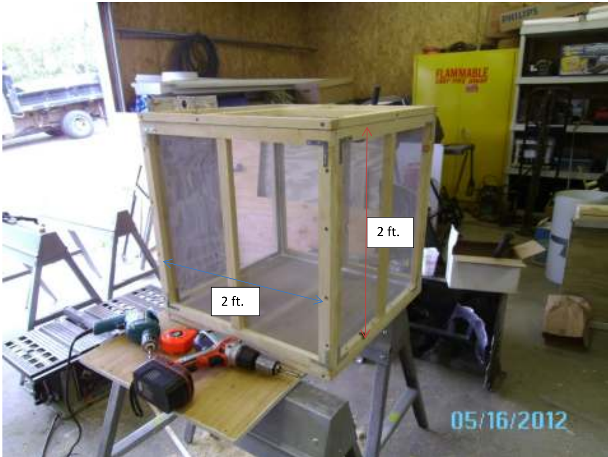
Holding pen showing slide gate and screen mesh.
