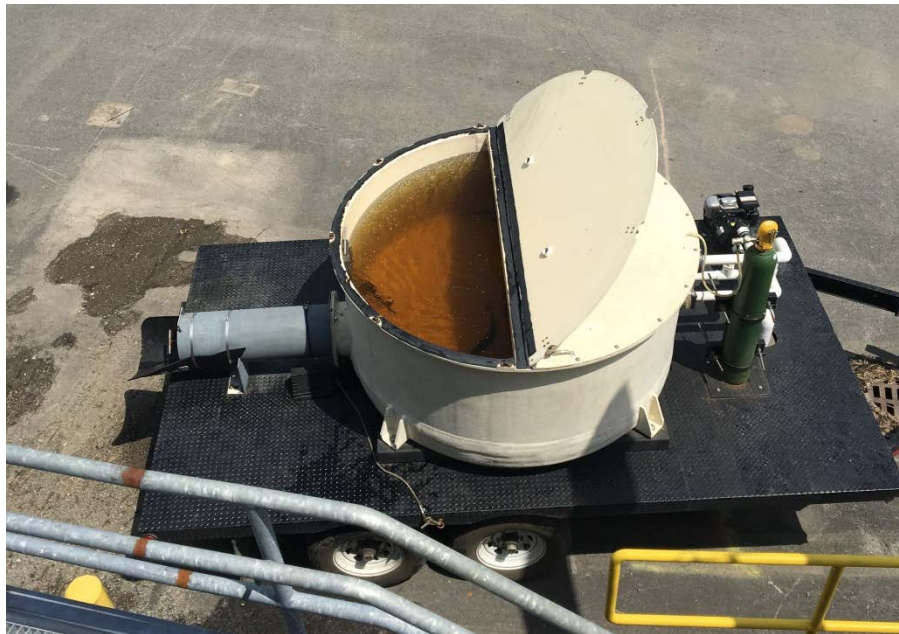
Figure 3.4-1. American shad transport tank used during tag and release efforts associated with Lower Penobscot adult shad outmigration evaluation.
