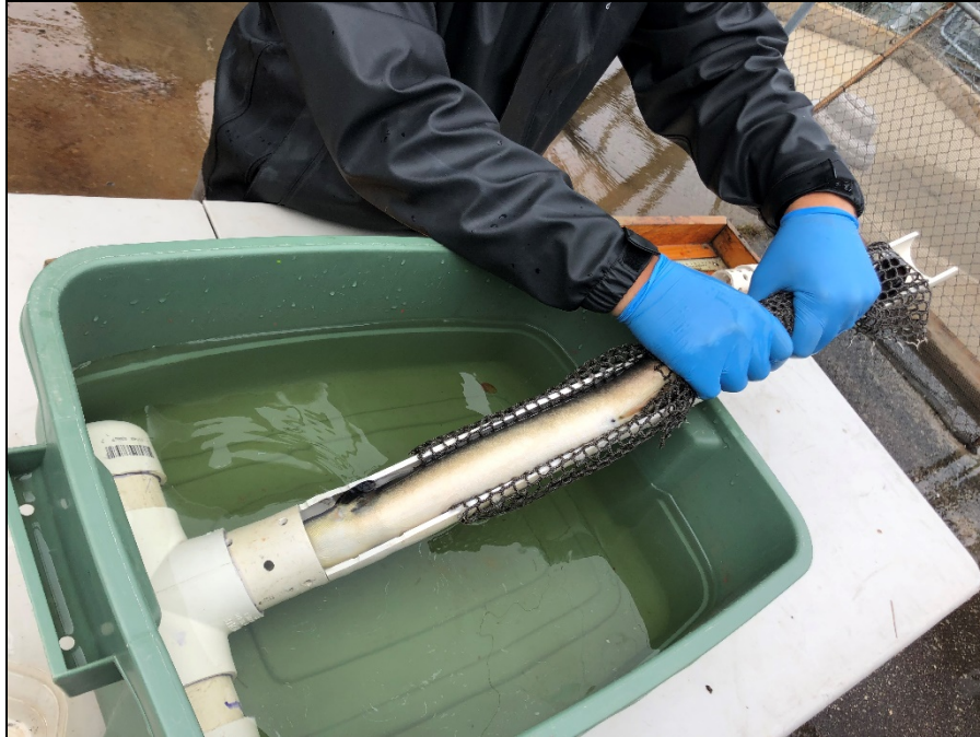
Figure 3–2. Restraint device for holding and positioning adult silver eels during radio-tagging.
