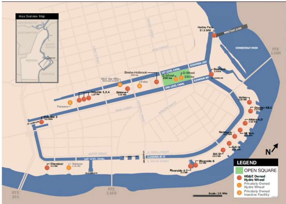
Figure 3. Dam and canal system layout. Open Square site shaded green. Flow enters canal system at upper right corner of schematic.
