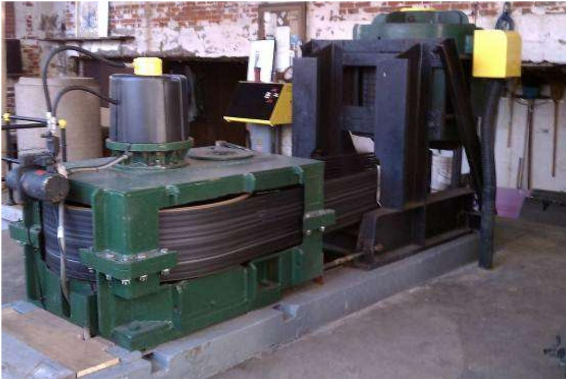
A belt driven Kaplan Turbine and Generator inside the Hydro Plant.
