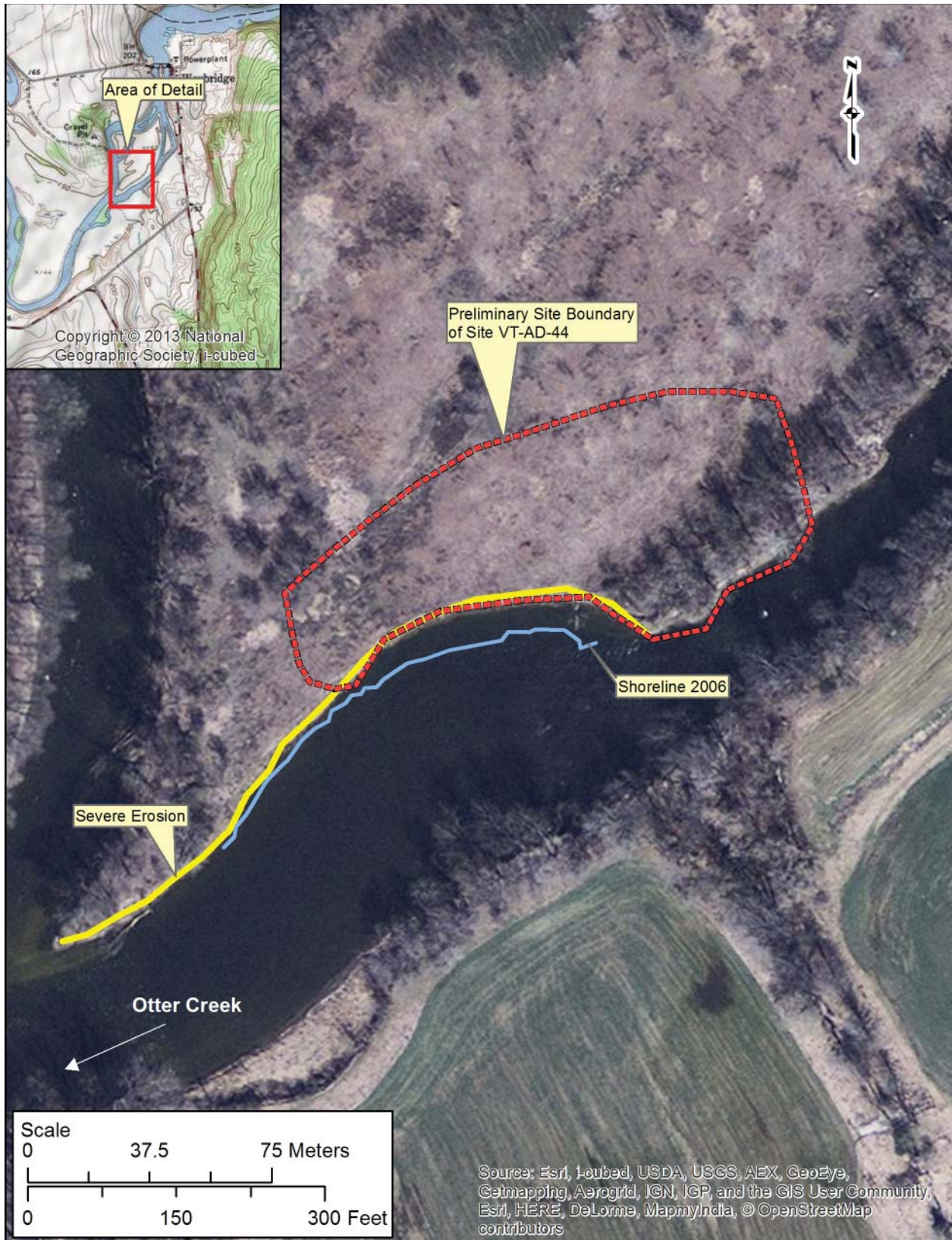
Figure 22. Aerial photograph showing areas of severe bank erosion at site VT-AD-44 within the Weybridge Hydroelectric Project (FERC No. 2731), Weybridge, Addison County, Vermont.
