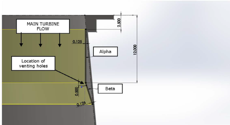
Fig 3. General parameterization of the aeration structure.
