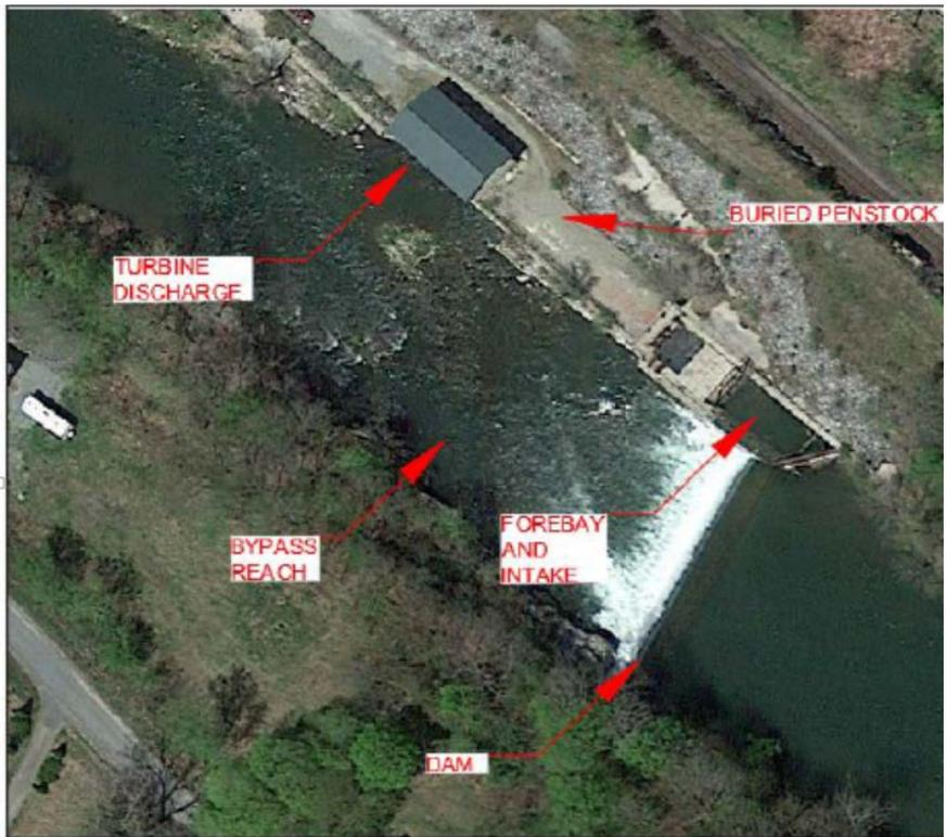
**Figure 2. Pownal Hydroelectric Project Site Overview.**
