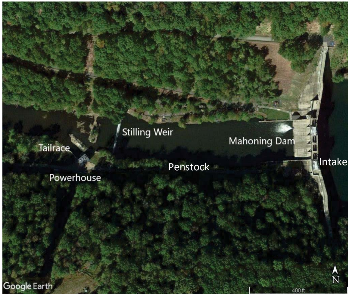
Figure 3. Google Earth Image Showing Project Layout and Key Features
