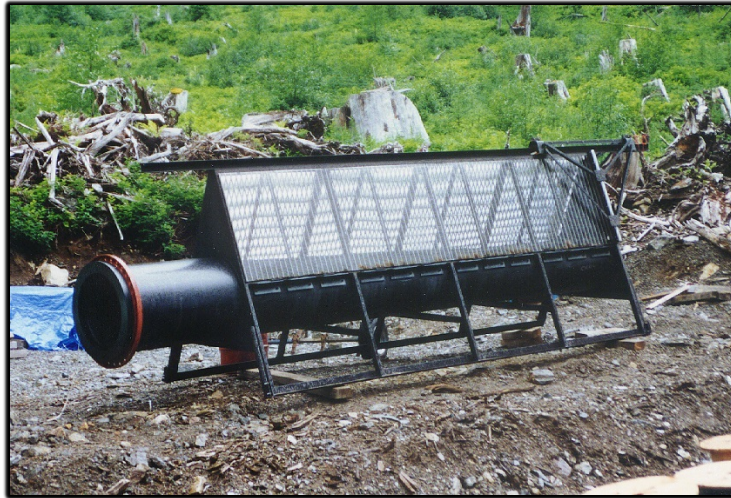
Figure 7: Wedge-Wire Screen Intake
