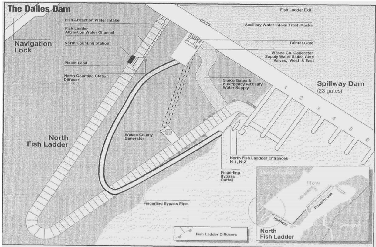
Figure 5. Northern Wasco County PUD Hydroplant Footprint
