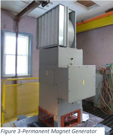
Figure 3-Permanent Magnet Generator
