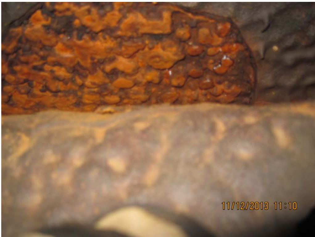
PHOTO 22 – CLOSE UP VIEW OF PENSTOCK NO. 3 DELAMINATION
