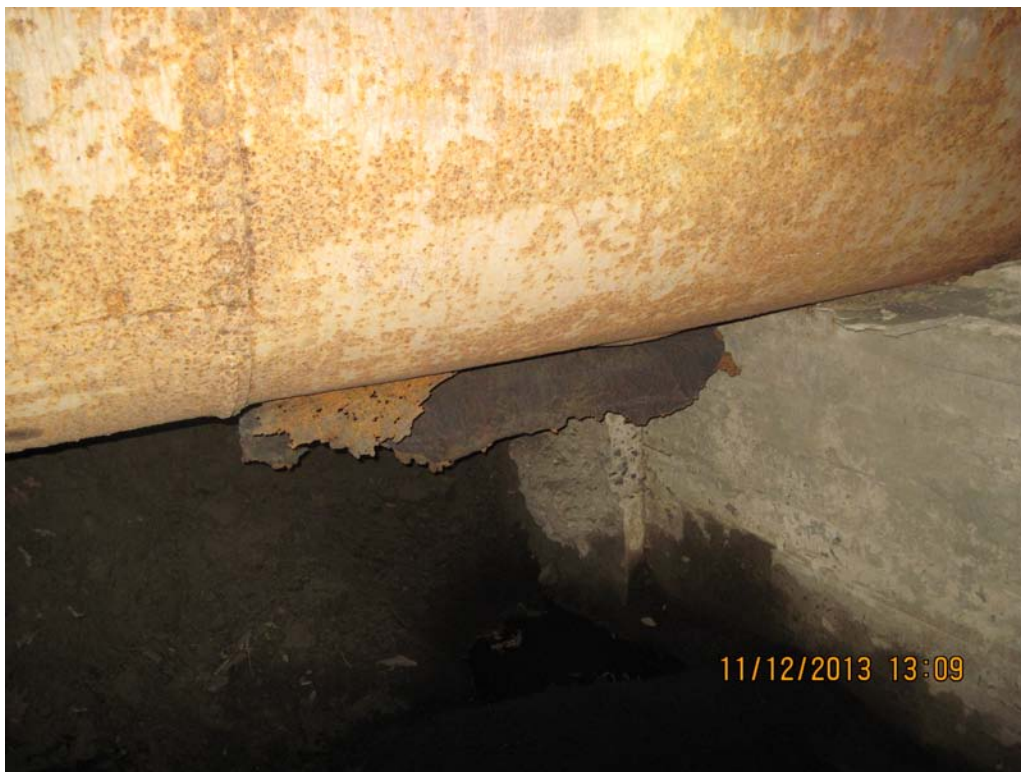
PHOTO 3 – EXTERIOR OF PENSTOCK NO. 2 FAILURE
