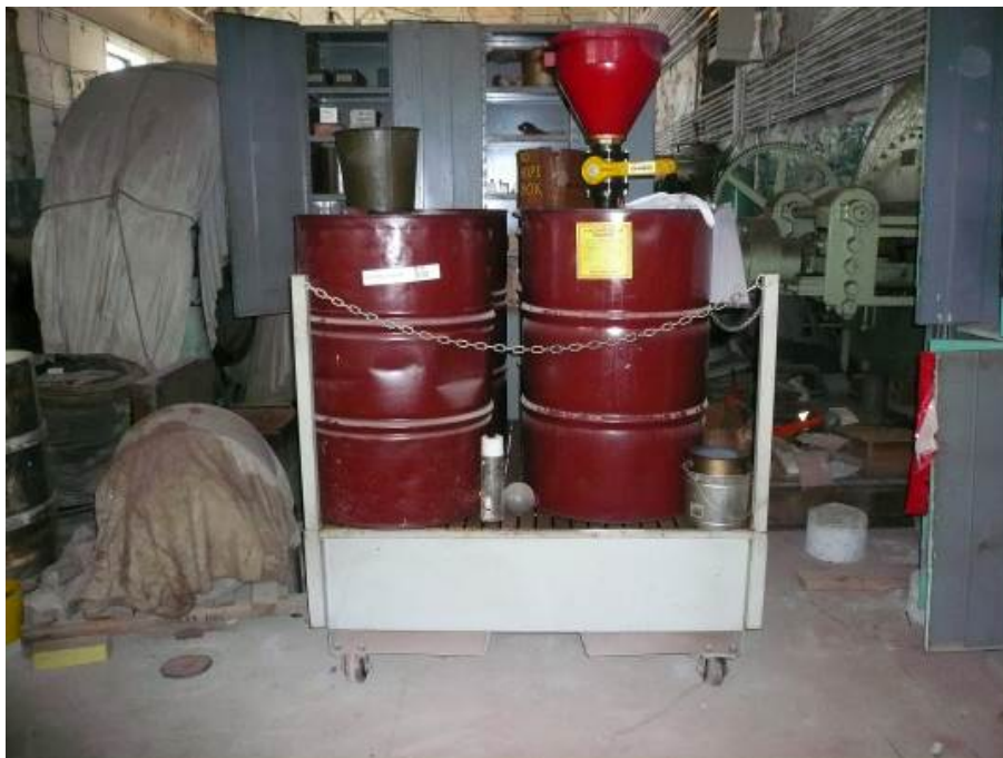
Photo 25: Secondary containment measures inside project powerhouse.
