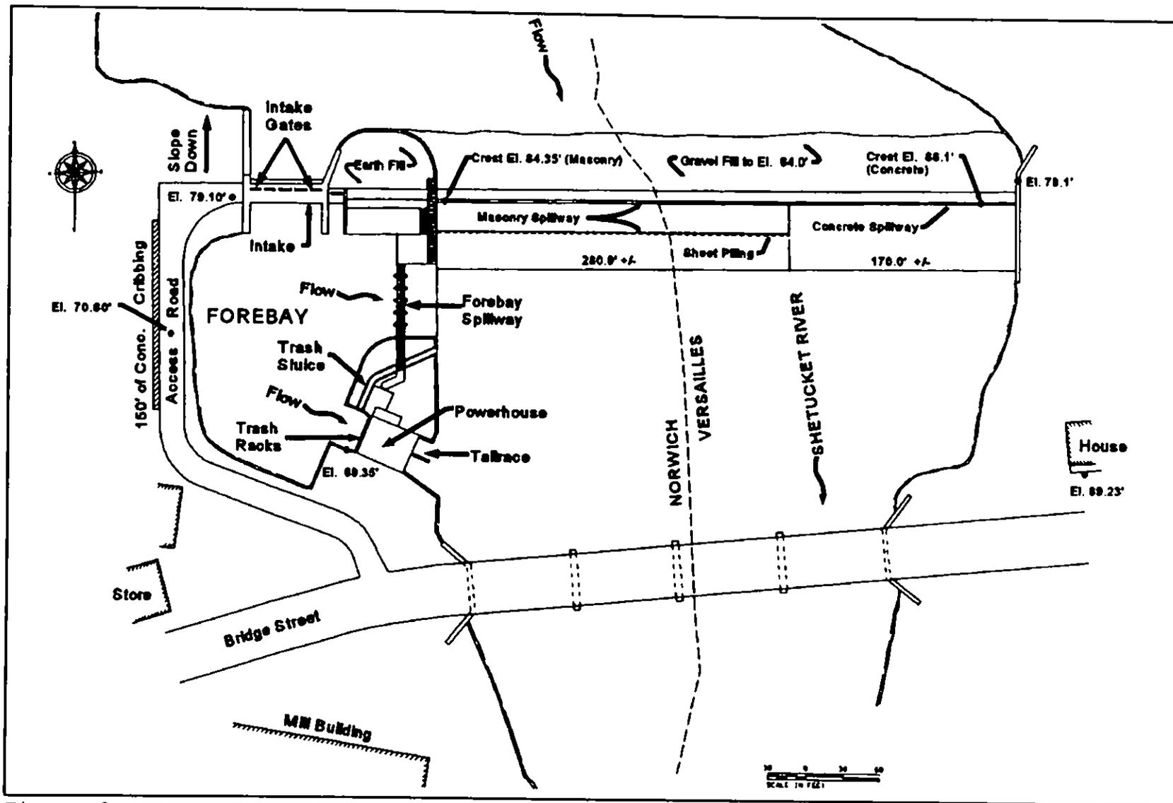
Figure 2. Occum Hydroelectric Project (Source: Norwich, 1996)
