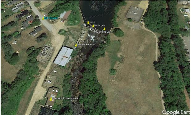
The FERC license requires a continuous minimum flow of 235 cubic feet per second (cfs) below the tailrace/powerhouse, or inflow to the reservoir, whichever is less, for the purpose of protecting and enhancing aquatic resources. A portion of the minimum flow, 30 cfs, is released at the dam, for the purpose of protecting aquatic resource in the bypass reach.
