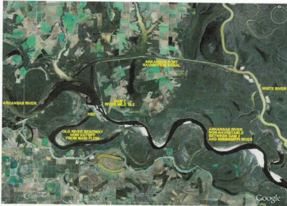
Satellite view of the McClellan-Kerr Arkansas Navigation System in the vicinity of the project. The Arkansas River and White River flow southeasterly to the Mississippi River (not shown in photo).
