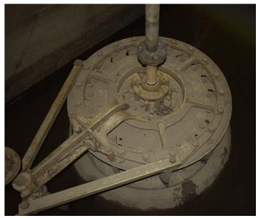
Figure 8. Leffel 27, B-4 propeller turbine (145 HP)
