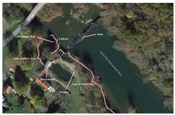
Figure 13. Overhead View with overlay of Site
