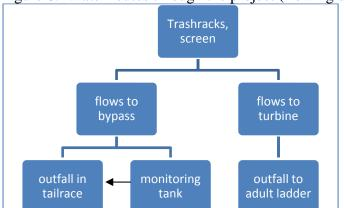
Figure 6. Water routes through the project (flowing down).
